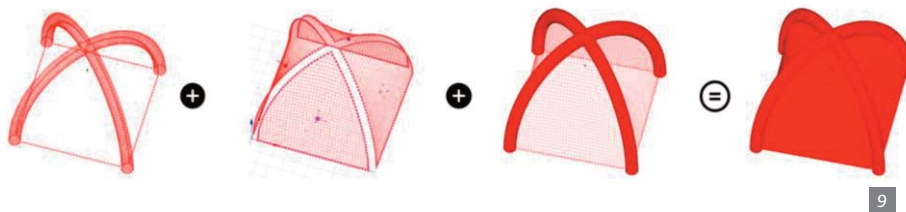
Figure 9. Sequence of the modeling with combined pneumatic and mechanical stressed structures.
